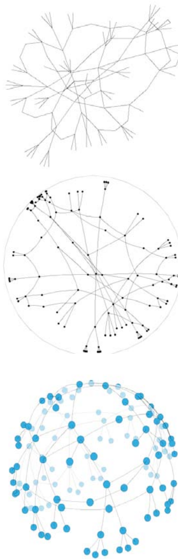
Figure 1: Drawings of the same simple, undirected graph obtained in Euclidean \mathbb{R}^2 space, hyperbolic \mathbb{H}^2 space and spherical \mathbb{S}^2 space. The graph has 121 nodes and 140 edges.
