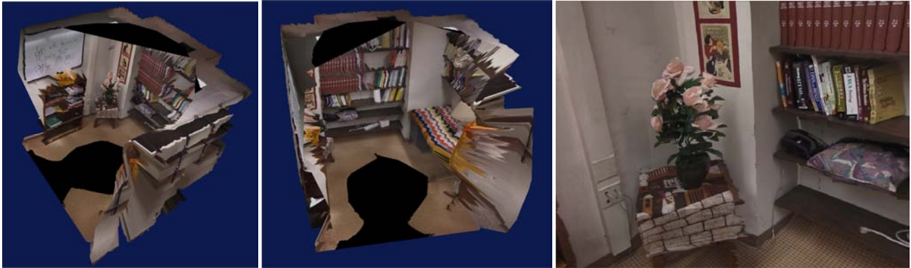
Figure 1 Depth enhanced panorama of a room: 100,000 triangles acquired in 30 minutes with a $3,000 device.
