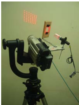
Figure 2 ModelCamera mounted in parallax-free pan-tilt bracket.
