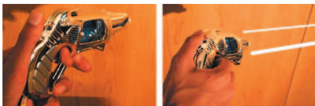
Figure 8: The raygun tool: Pressing the menu button (right) displays the two current options for the gun: drawing Phosphate bonds (thin line) and drawing Hydrogen bonds.
