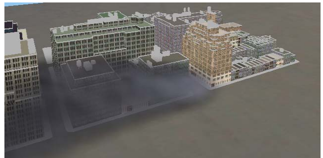
Figure 7: Snapshots of smoke dispersion simulation in West Village area of New York City at time steps 247, 288 and 319.
