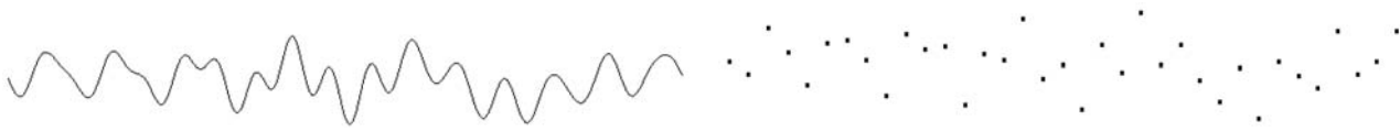
Figure 4: Left: original continuous signal with 19 frequencies. Right: a set of samples sampled at the Nyquist frequency, the number of samples is 38.
