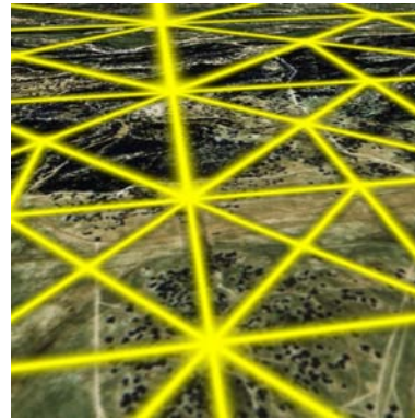
Figure 1: Two screen shots of an overflight of Fort Hunter Liggett, CA that illustrate the use of 4-8 texture hierarchies. On the left is the seamless textured image produced by the system, while the right shows the outline of the texture tiles used in producing the image.
