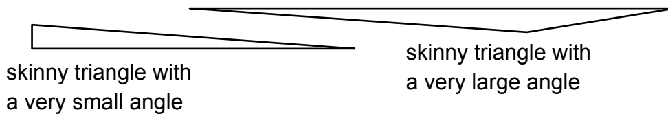
Figure 2.2.1. Examples of poorly shaped triangles
